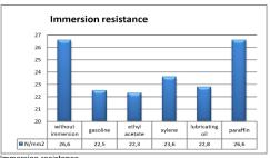
The samples were immersed in various fluids for a period of 90 days at 23 ° C. Afterwards the samples are tested a shear strength till the adhesive breaks. A comparative study is made with a sample without immersing Test. Curing time: 16 hours at 40 °C and immersion in each fluid during 90 days at 23 °C
